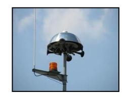
The THORGUARD sensor continuously monitors the atmosphere's electrostatic energy and evaluates the potential for lightning. When the system determines a hazardous condition, theair-horns and strobe light provide necessary alerts.
